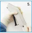
Pinch new tubing and press into channel on top rear of the handpiece. Pull tubing forward and down handpiece firmly. Pull tubing to the rear or cut so tubing is flush with distal end of handpiece.
